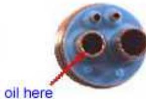
**Weekly:** Additional lubrication should be applied to inside nose of motor.
