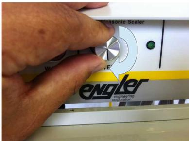
To enable the ultrasonic scaler, locate the power switch on the front of the control unit, (see photo) Turn the knob clockwise. The LED will illuminate indicating that the scaler is ready for use. This not only turns the unit on, it also allows the operator to precisely adjust the power setting of the scaler from minimum to maximum.
