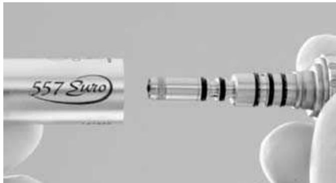
4. With bur engaged, operate handpiece to expel excess lubricant. Wipe off any excess lubricant with a towel or cloth.
