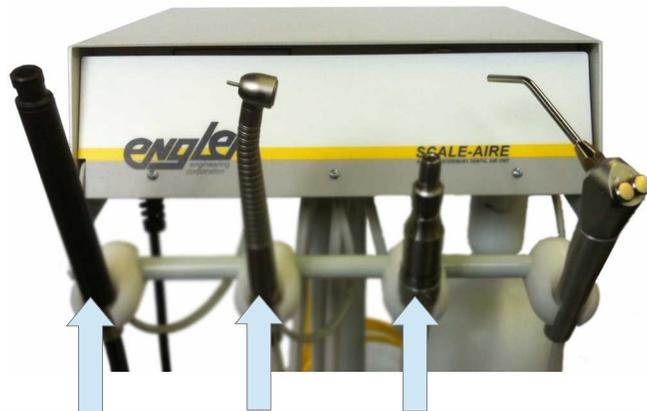
The Scale - Aire has three automatic handpiece activators. Each handpiece must go into its corresponding activator. The order from left to right is; ultrasonic scaler handpiece, high speed handpiece, and low speed handpiece. Select the desired handpiece by lifting it out of its holder, the Scale-Aire will automatically select THAT handpiece for operation.
