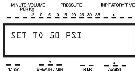
e. To exit this mode, simply release the FILL & HOLD button and the unit will go through the self test.
