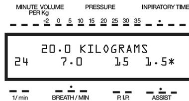
**NOTE:** An "\*" is displayed as an indication that the A.D.S. 1000 is in the PEEP mode.
