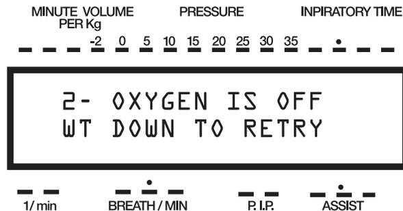
This may indicate a number of problems. In order to test all internal lines and valves the A.D.S.1000 attempts to pressurize itself and then checks for leaks. If it cannot pressurize itself then it will give the above readout. The causes for the error are as follows:
