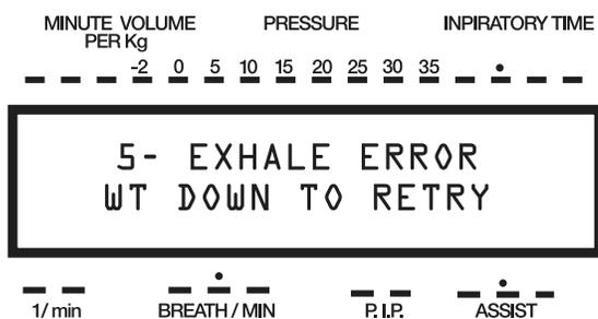
This display indicates that there is an obstruction to the exhale valve or that the exhale valve did not open. This error can be caused by the following.
