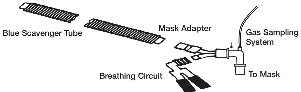
4. Connect the external sensor input - insert the Luer lock connector to the gas sampling input and rotate it clockwise one half turn. Now insert the gas sampling elbow into the end of the mask adapter.
