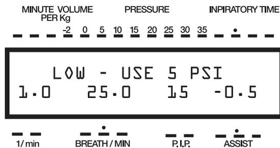
3. On the back panel of the A.D.S. 1000 you will find a toggle switch to select the pressure - 50 P.S.I. for normal operation (and to start up self test) and 5 P.S.I. for lab mode. Set switch to 5 P.S.I.
