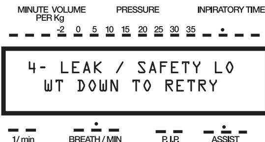
This display indicates that there is a minor leak or the Safety pop-off is releasing at too low a pressure.
