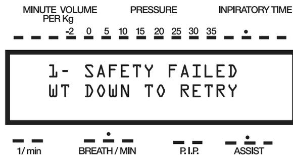
This indicates that the mechanical Safety pop-off valve inside the unit is dirty or it has failed.
