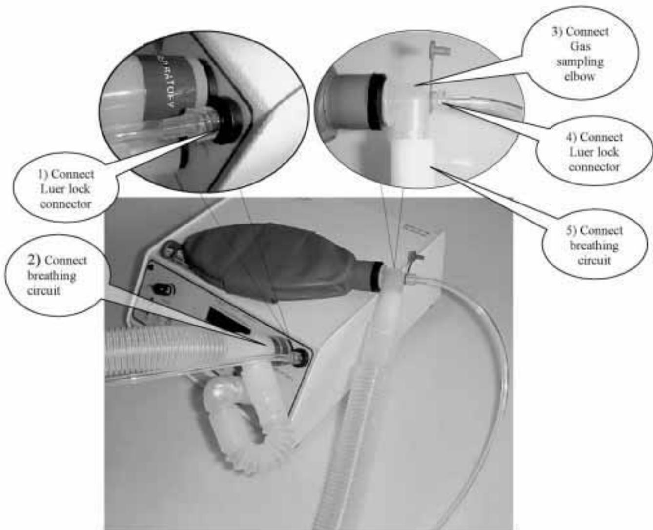
**Note: Do not connect test lung until unit has been properly initiated.**
