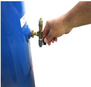
Once all of the O2 has been vented from the tank, the gauge should read 0. Disconnect the hose underneath the control box leading to the tank.
