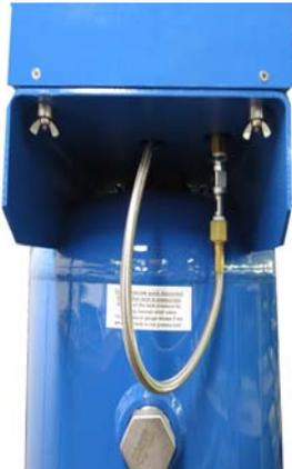
Carefully lift the blue control box off of the tank and place in a well padded box for return to EEC. Pay special attention to prevent damage to the screws at the bottom of the blue box.
