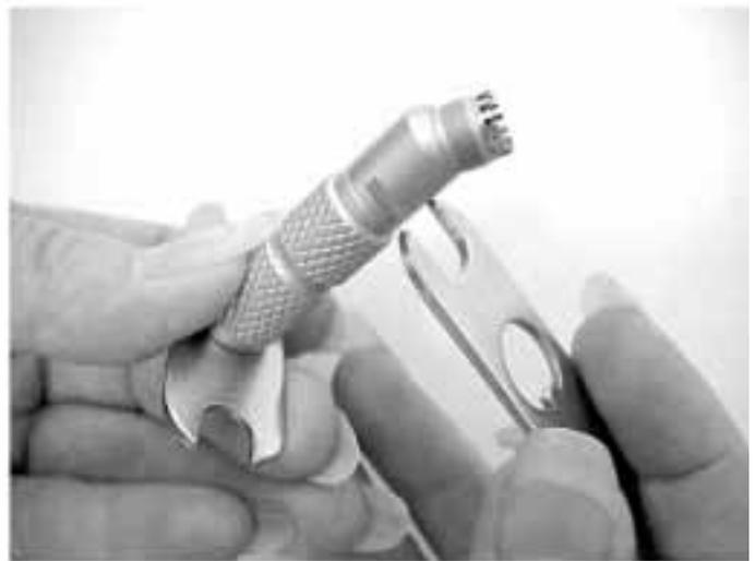
TO SEPARATE MIDDLE BODY FROM MAIN BODY POSITION THE WRENCHES AS SHOWN. TURN WRENCH IN FIGURE B COUNTER CLOCKWISE (DO NOT MOVE LOWER WRENCH.)
