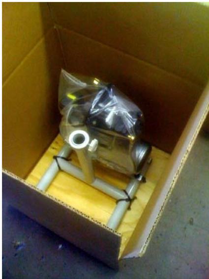
All four sides of the frame should be secured.
