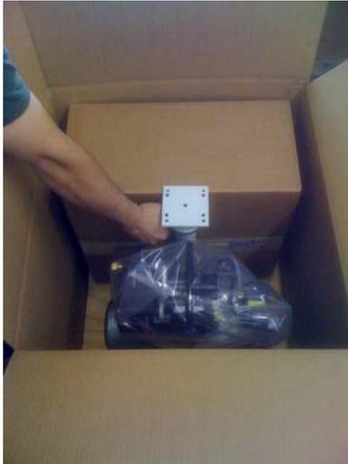
Reinsert the adjustable post and tighten. Note that the flange helps hold the small box in place.
