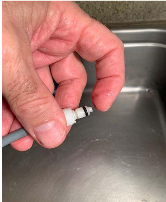
When you push the nipple in, water should shoot out in a strong stream. If it doesn't, the pump is not pressurized enough or there is some other obstruction (clogged filter or water source?).
