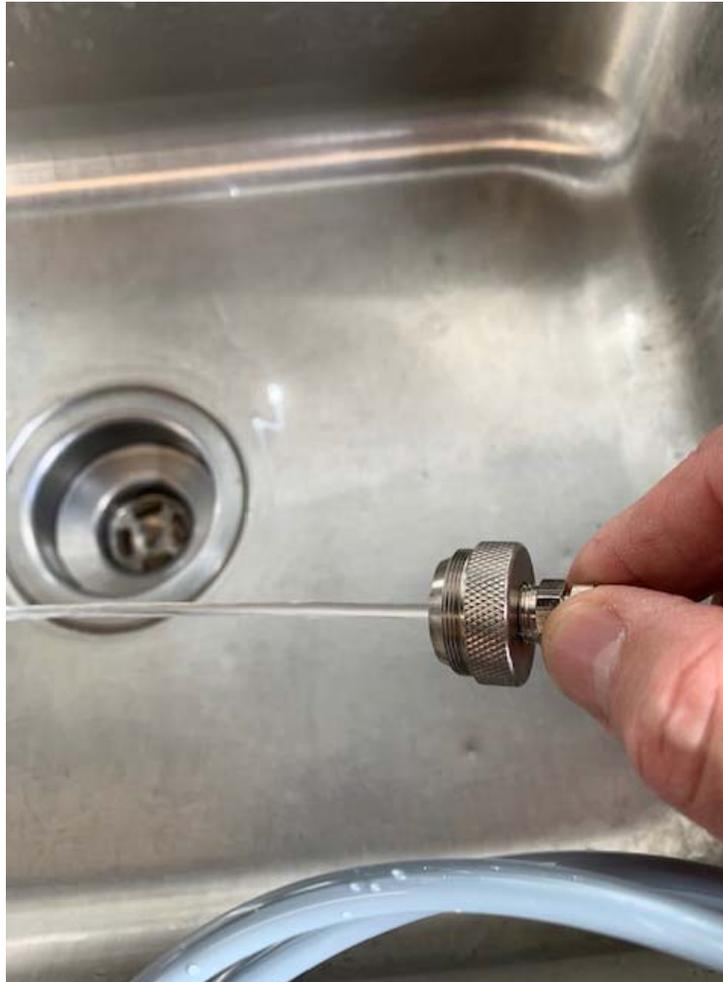
To confirm that water is flowing up to the unit, disconnect the waterline from the back of the unit by pressing the stainless steel tab (shown on page 5).
