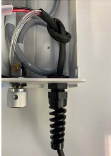
This photo shows the cable passing through the strain relief at the front of the unit, a 1 to 2 inch lead, then a loose knot. The knot is there to prevent the cable from detaching from the circuit board causing an unsafe electrical hazard.
