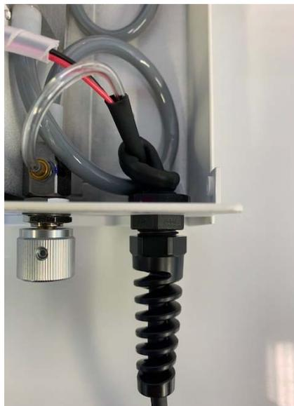
This photo shows that the Handpiece Cable has been pulled far enough that the knot is tightening against the inner wall of the scaler, possibly choking off the water flow.
