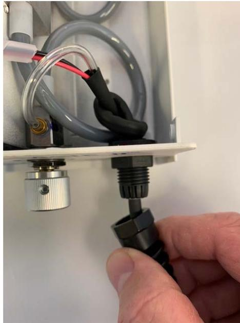
Start by loosening the Strain Relief. Once loose enough, push the cable back into the unit. It only needs to go back 1 to 2 inches.
