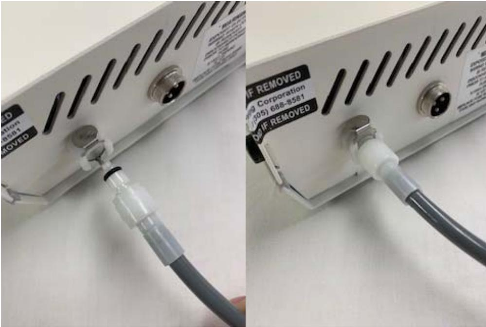
The photo on the left shows the Male Q/D is intact and is about to be inserted into the unit. The photo on the right shows the Male Q/D properly connected.
